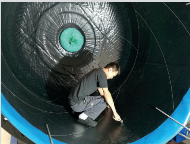
Fig 13: Stitching tire cord layers manually. The shoes used for stitching the rubber sheets are dedicated only for this operational process to prevent any risk of contamination.
