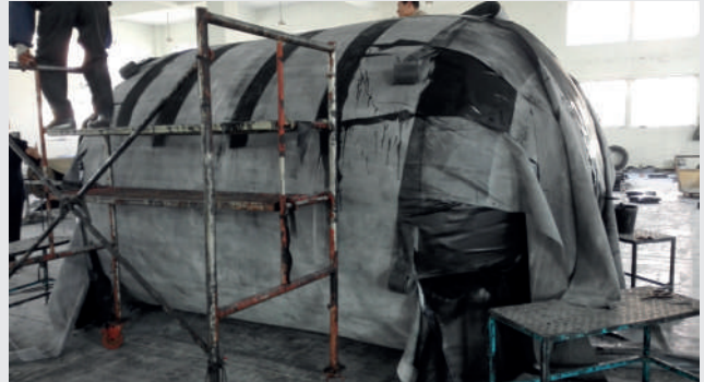
Fig 14: Tire cord layers are applied on the bladder at 90°
