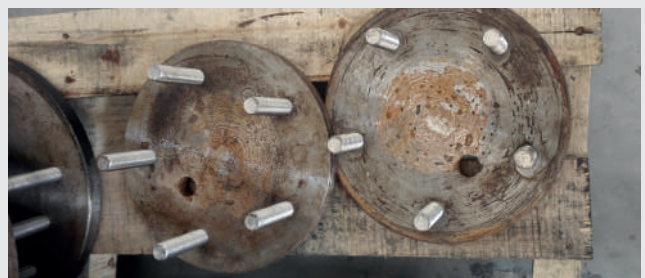
Fig 15: Inner Flange – a simple construction
