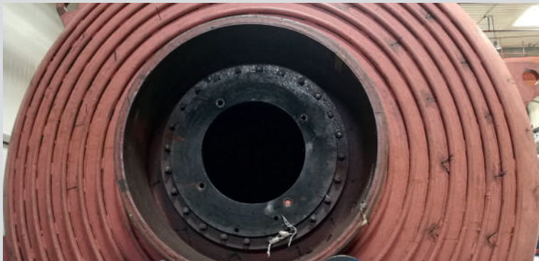
Fig 9: Side view of a mold showing the flange opening
