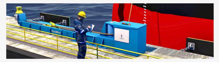
The next generation of mooring systems, DynaMoor, combines Trelleborg's class leading Quick Release Hooks with an innovative dynamic tensioning system.
