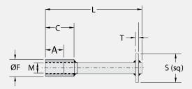
Always check min/max clamping thickness and socket depths actual threaded length on bolts.
