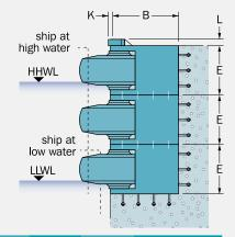
The table indicates typical Wheel Fender casing dimensions. For special applications and unusual corners, the casing shape can be altered for a perfect fit. Please ask Trelleborg Marine Systems for details.
