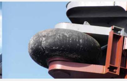
Roller fenders are usually installed to guide ships in restricted spaces like walls of dry docks.
