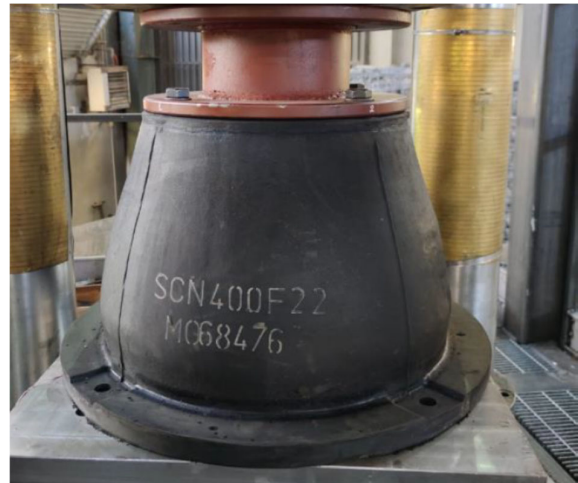
Figure 2: Cone fender undergoing cyclic compression testing (Politecnico Milano)
