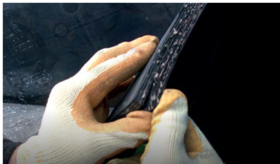
Figure 16: Delamination of wrapped pneumatic fender in between reinforcing tire cord layers.
