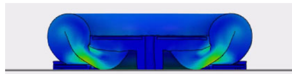
Figure 9; Stress development example (FEA) in a cone fender (Trelleborg)
