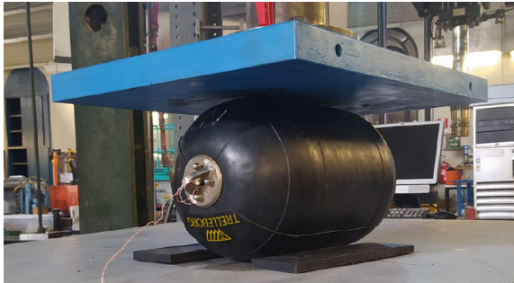
Figure 12: Cyclic testing of a Pneumatic fender (Politecnico Milano)
