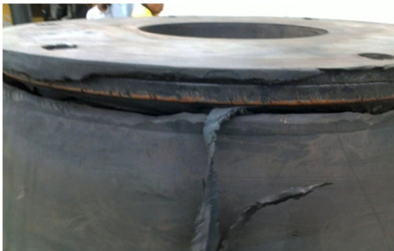
Figure 11: Debonding of the embedded steel plate (Port in South east Asia, fenders from a local manufacturer)
