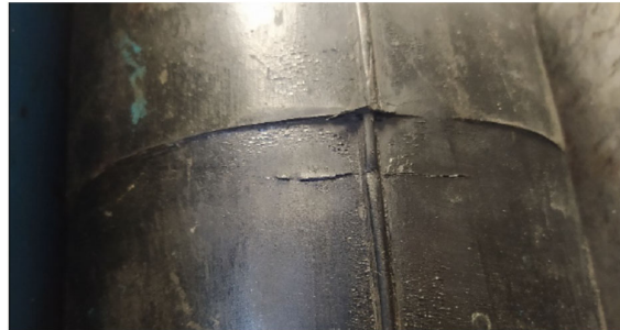
Figure 15: Fender body after 250K Cycles (Politecnico Milano).
