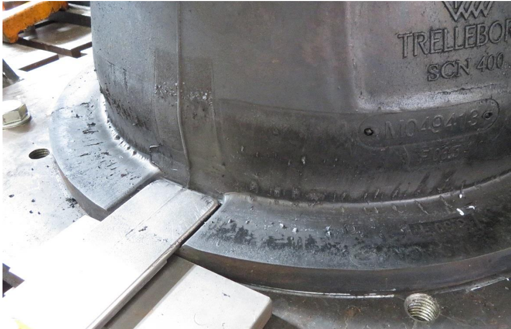
Photo 8- Small rubber deposits seen on the flange
