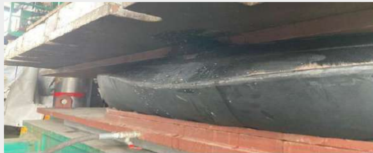
Figure 9. Failure mode at 80 mm compression at 5.8 bar
