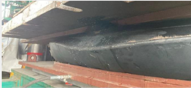
Figure 9. Failure mode at 80 mm compression at 5.8 bar
